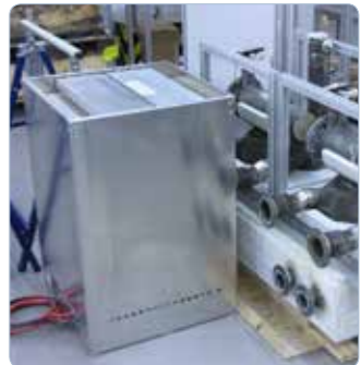
Part of the SOFC lab setup with one of the two 5 kW modules
