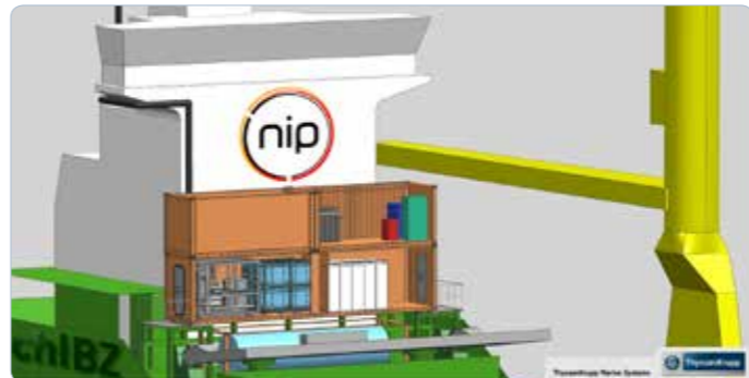
CAD representation of the experimental setup with a hybridized 100 kW SOFC system on board of MS Forester
