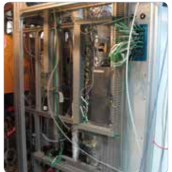
Front view of laboratory diesel reformer for the test with two 5 kW SOFC modules
