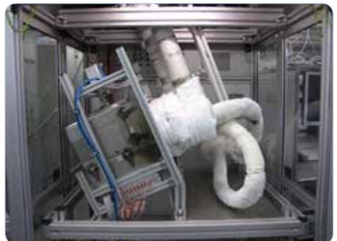
Test of a SOFC module on maritime capability (inclination, vibration)
